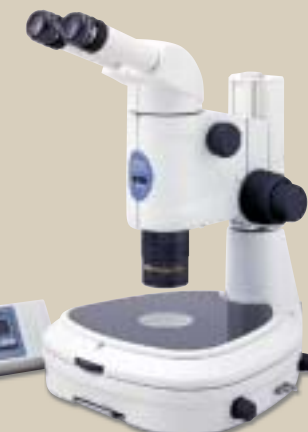
Thermo-plate made by TOKAI HIT mounted on SMZ1500.
