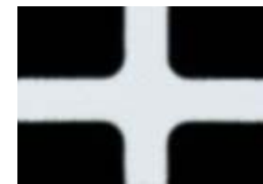
A cross line in the viewfinder makes for easy manual focusing.
