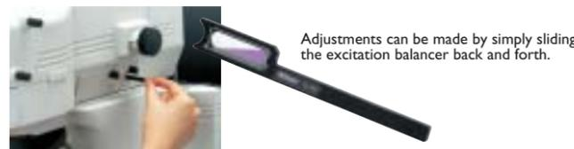
Adjustments can be made by simply sliding the excitation balancer back and forth.
