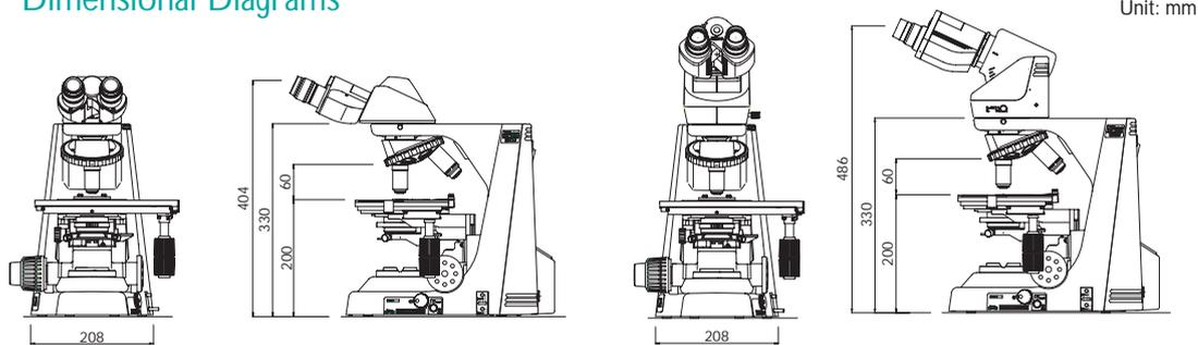
Configured with binocular tube B
