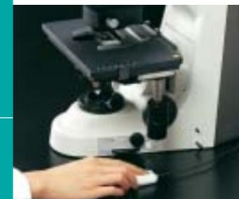
Marking is easily performed while observing the image. Quick-dry ink facilitates fast, clean marking.
