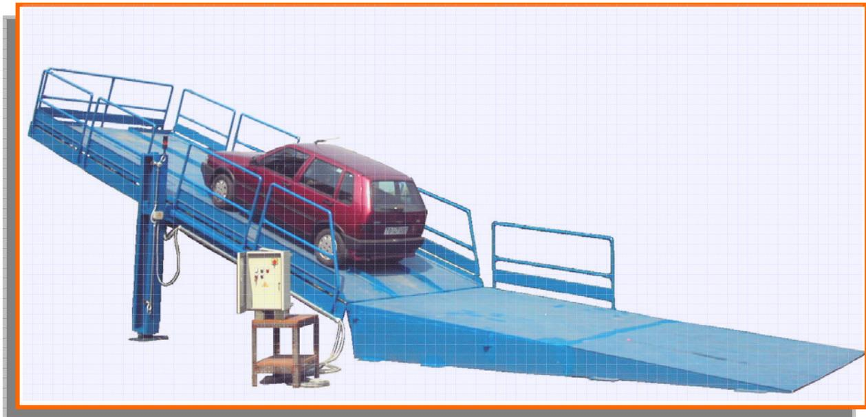
**Sloping Ramp** represents a cheap and effective method for testing long term efficiency of vehicle's parking brake. Further, this equipment requires a **very little maintenance** and, due to its simplicity, has a **long time reliability**.
