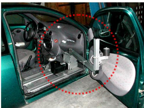
**The Inside Bench** is to be mounted at the place of a seat and open and close a door according the same program as the outside bench, it open with different speed pushing a door and it close the door by a rope linked to the door itself
