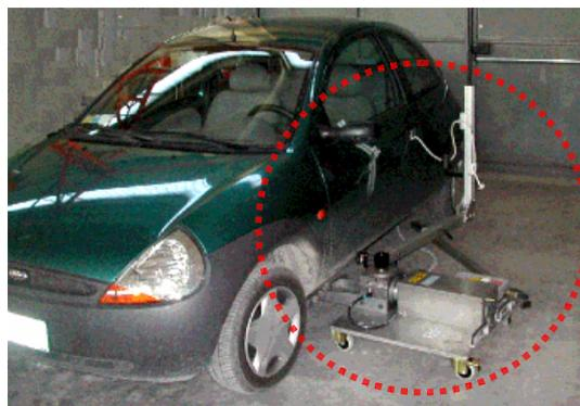
**The Outside Bench** is very compact to work also with cars very low, it is locked to the car frame, customers should point out the minimum and maximum height of the cars they want to test.
